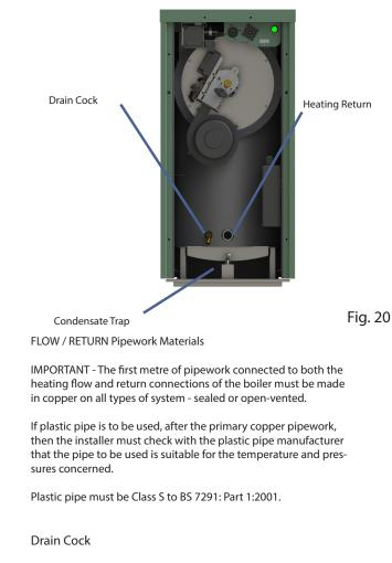
A drain cock is pre-fitted to the boiler. (See Fig 20)
