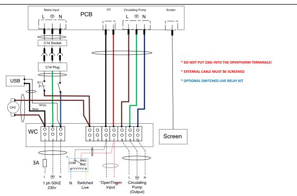
Internal Wiring Diagram (Sapphire PCB Connections)
