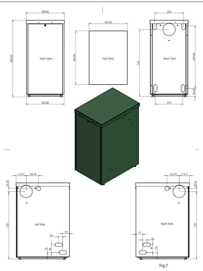
ALL DIMENSIONS IN THE DIAGRAMS ABOVE ARE IN MILLIMETRES
